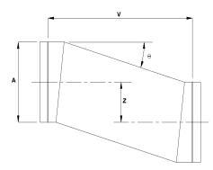
Note: Z should not exceed 0.75A or  $\theta$ >60°. If larger, use fabricated elbows and a straight length of duct.
