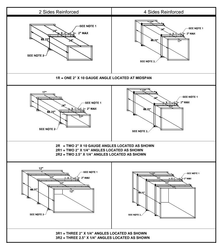
Table 13 Reinforcement for 6-Foot Joints Using External Angle (continued)
