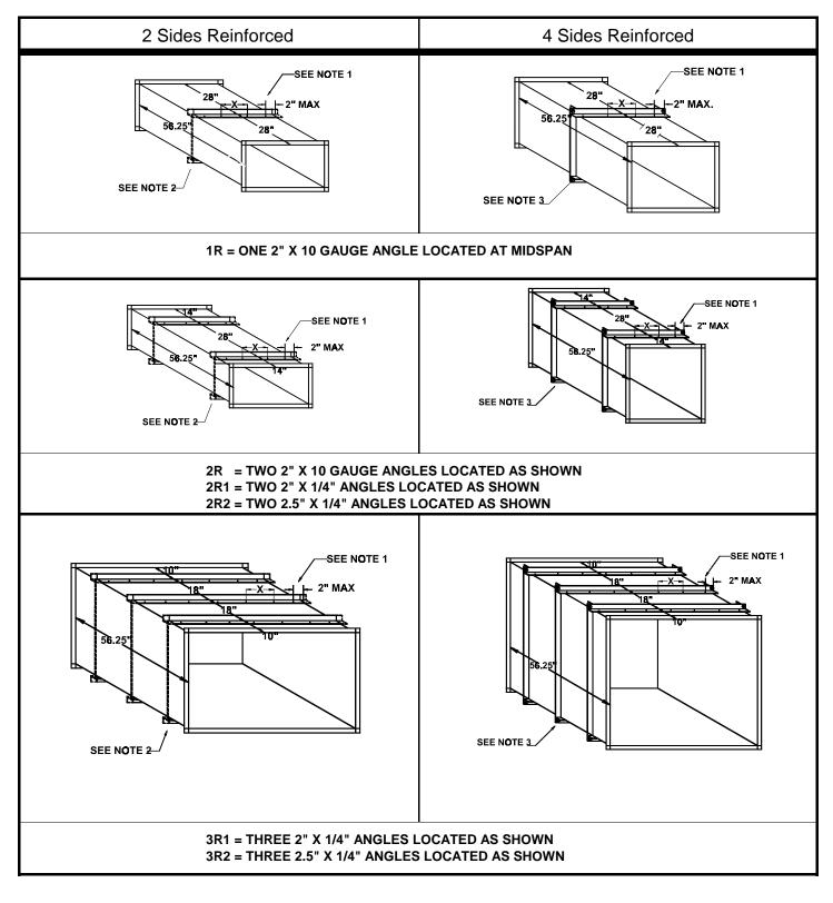
Reinforcement for 5-Foot Joints Using External Angle (continued)
