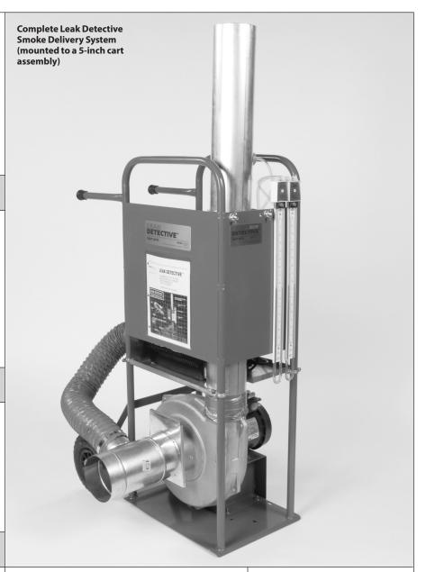
The expected accuracy of all our orifice tubes at the time of shipment is 2 percent of the indicated flow rate. All tubes are supplied with calibration charts and tables certified by a professional engineer (see Figure 1).
