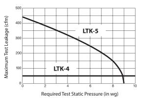
Figure 3 CFM versus Test Static Pressure
