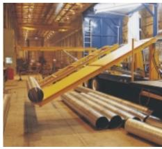
Each Mobile Duct Machine uses a pneumatic or hydraulic handling table, which allows the operator to deliver the duct directly into the hands of the contractor.
