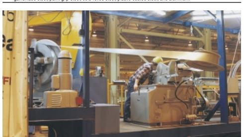
Each self-contained Mobile Duct Machine is equipped with an air compressor, welding machine, steel decoiler, heating, and lighting. A separate truck-mounted electrical generator is also available.
