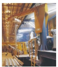
Each mobile unit is equipped with a 2-ton overhead crane for easy and convenient material handling.
