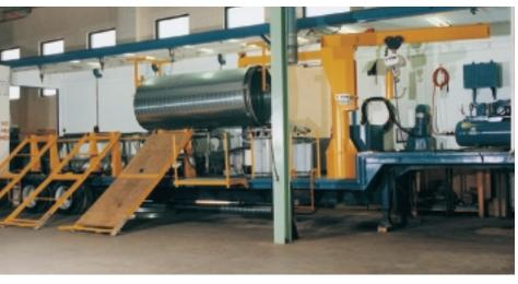
McGill's Mobile Duct Machine is a self-contained, 42-foot trailer with an air compressor, welding machine, steel decoiler and a two-ton, overhead crane. A pneumatic handling table delivers the duct directly to the contractor.
