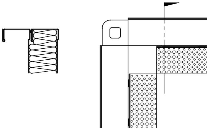
**Note:** For thicker insulation, additional nosing is tacked in place between the inner and outer TDC flange or the inner flange is left unformed and used as nosing.
