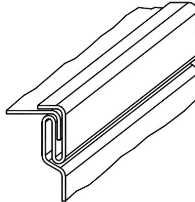
Double-wall k27 Duct Construction
