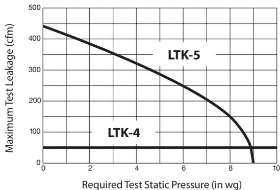
Figure 3 CFM versus Test Static Pressure
